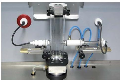
Fig. 3 Apparatus for determination of minimum ignition energy of a dust/air mixtures (Anko, 2015)
