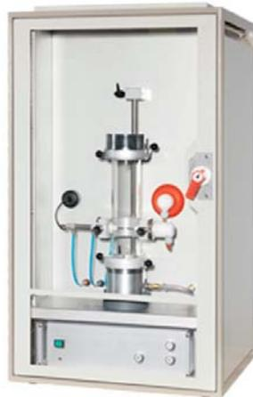
Fig. 1 Minimum Ignition Energy Apparatus (MIKE 3) (Kühner safety, 2015)
