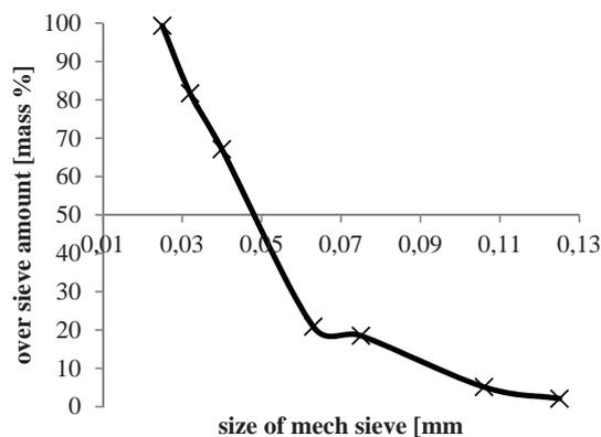
Fig. 5 Grain size analysis - Powder paint
