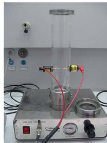
Fig. 2 Minimum Ignition Energy of a Powder Test Apparatus (MIE III)
