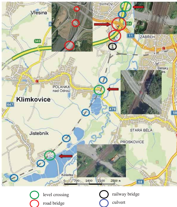
Fig. 3 Map of selected hazards on the railway route with marked critical points
