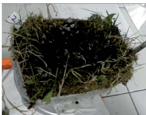
Fig. 4 and Fig. 5 Sorbent LITE-DRI applied on samples of arable and grassy soil after 1 minute of motor oil contamination
