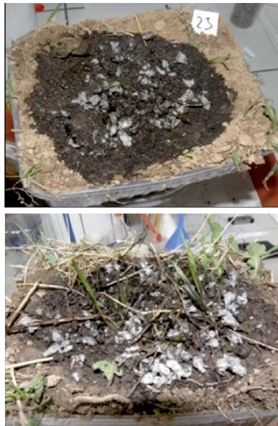
Fig. 8 and Fig. 9 LITE-DRI sorbent applied on arable and grassy soil sample after 30 minutes from motor oil contamination
