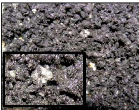
Fig. 3 Sorbent LITE-DRI soaked with motor oil
