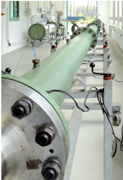
Fig. 4 Instrumented experimental pipe to investigate detonative properties of gas mixtures. Diameter 200 mm, length 30 m, max. pressure 40 bar
