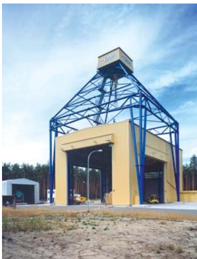
Fig. 7 Drop test facility (200 tons lifting capacity) on BAM TTS
