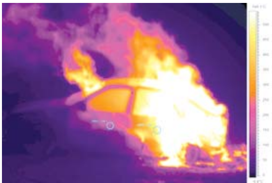
Fig. 9 Photograph of a car and a thermogram of the car body surface. At the measurement points marked on the thermogram, the average temperatures were: 158.1°C and 495.7°C
