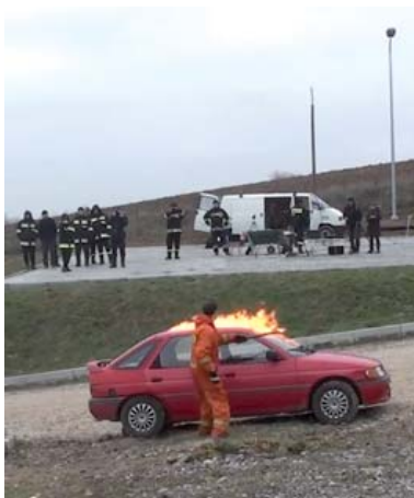
Fig. 4 Setting the Ford Escort car on fire. The measurement stand in the background
