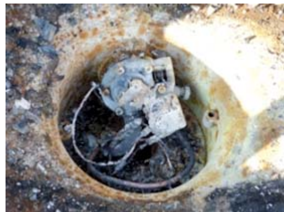
Fig. 2 Multivalve of the LPG tank before and after combustion
