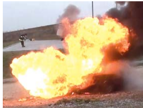
Fig. 6 Ignition of gas released from the LPG tank
