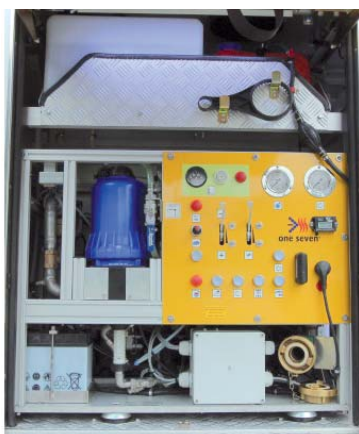
Fig. 3 Vehicle with single hose line and streamline - left, compressor and proportioned One Seven OS-C0-100-MR - right
