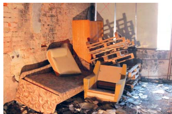
Fig. 2 Disposition of combustible material in the test room
