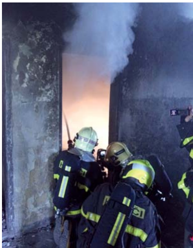
Fig. 5 Application of compressed air foam into the examination room
