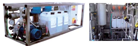
Fig. 5 Mobile versions of water treatment (MSRO 140, SVK - MÚPV 5)
