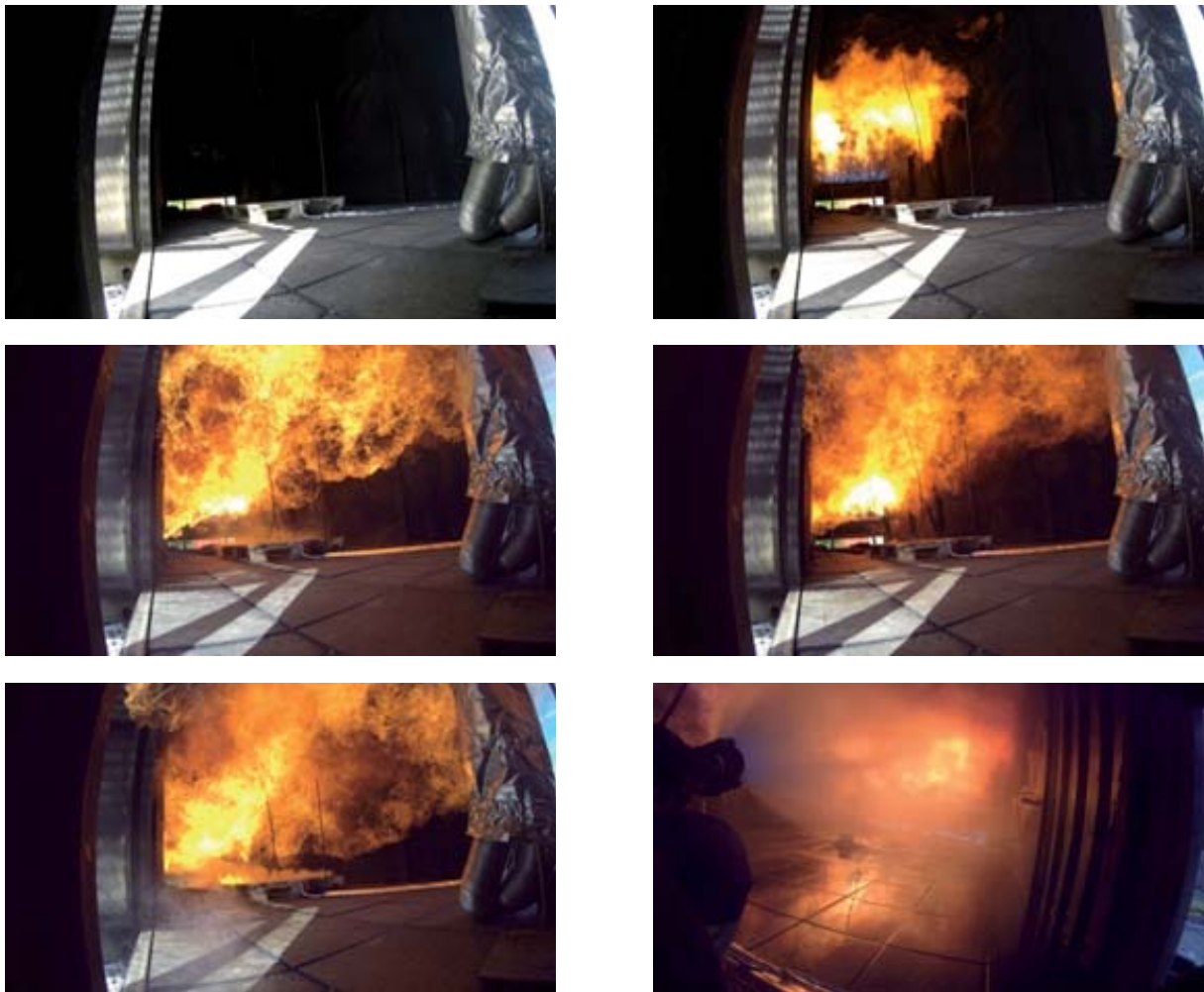
Fig. 3 to 8 Conditions inside chamber 1 during measurement with water supply
