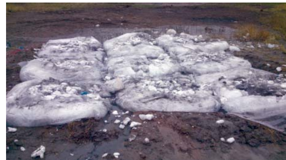
Fig. 27 Test result – the fragmentation of ice blocks
