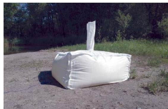
Fig. 14 and 15 Photo of the developed textile sealing bag with a volume of 250 and 500 liters of water
