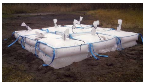
Fig. 26 Field tests of charges on artificially created ice blocks
