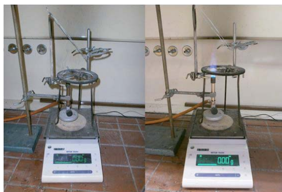
Fig. 3 The testing device for fire tests constructed and located in the Fire-chemical laboratory of the Department of Fire Engineering, FBI, University of Žilina
