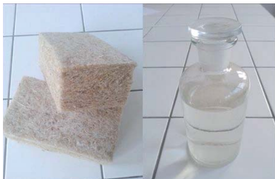
Fig. 1 The representative picture of thermal insulation product Canabest Basic and the representative picture of fire retardant Ohnostop Special
