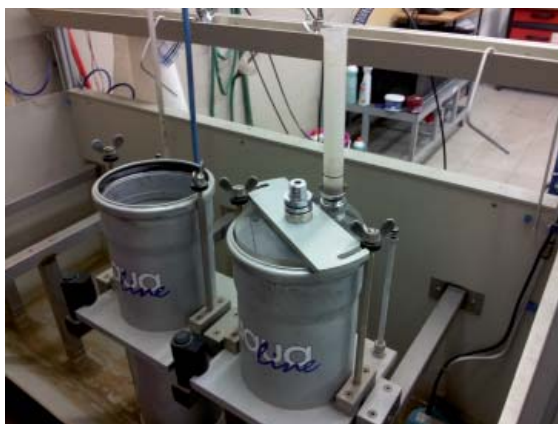
Fig. 7 Test device for hydraulic pressure test and for the test of volume expansion of PCs at Repair plant of FRS CR in Olomouc
