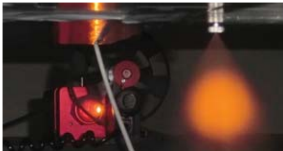
Fig. 13 Detail of dispersed radiation on water droplets
