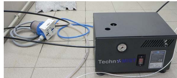
Fig. 2 High-pressure pumping unit with supply line and filter
