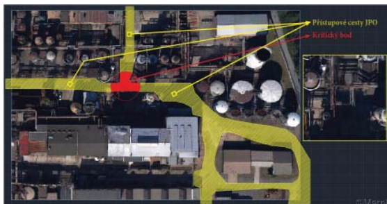
Fig. 7 Industry plant analysis - access roads in yellow, critical point in red (Marek and Nejtková, 2017)
