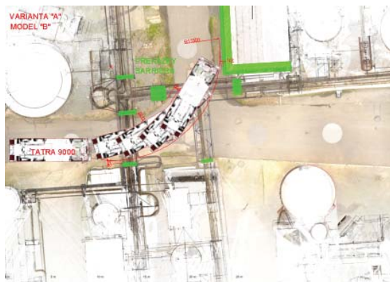
Fig. 13 Fire engine passage simulation outcome: Variation passage A to C, model A with no skid or trace correction (Marek and Nejtková, 2017)
