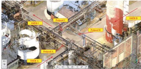
Fig. 8 Detailed, real and accurate spatial coloured model of entire situation (Marek and Nejtková, 2017)
