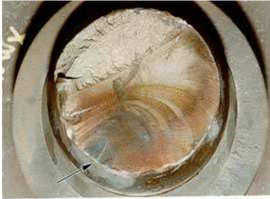
Fig.4.: Fracture surface of the axle of the railway bogie [7]
