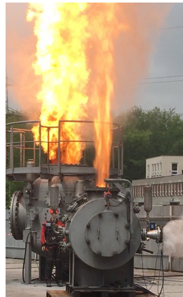
Fig. 1 Example of flame transfer in vessels connected by piping during explosion tests
