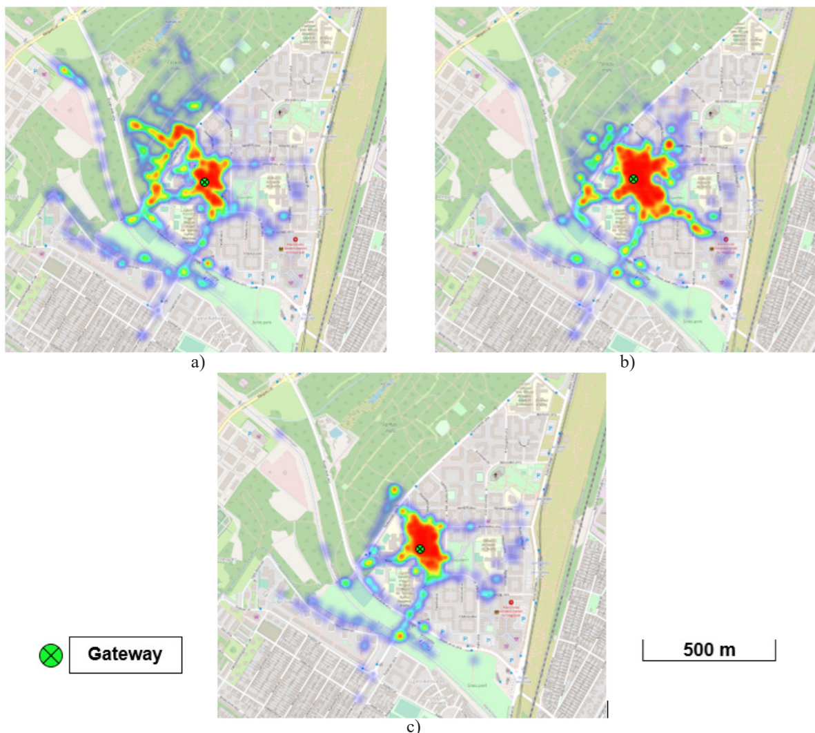
Fig. 2 Mikrotik Gateway; a), Tracknet Gateway; b) and Kerlink Gateway; c) RSSI heat map
