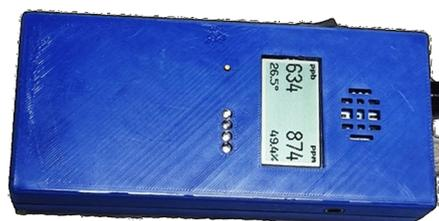
Fig. 5 Designed and constructed portable ozone detector
