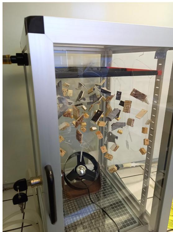
Fig. 1 Samples of materials prepared for ozonation
