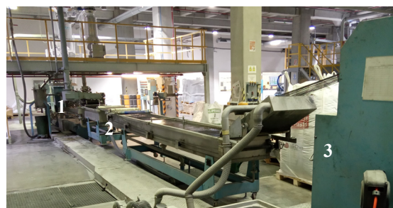
Fig. 1 Production line for polymer processing (1 extruder, 2 cooling bath, 3 pelletiser)
